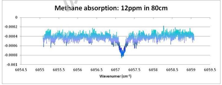
Example of 12ppm concentration of methane in 80cm flowcell. Simulated using HITRAN methane data and actual scanned cell data. Used Agilent 8164A tunable laser to scan line. 0.02% is roughly the noise floor of the laser.
